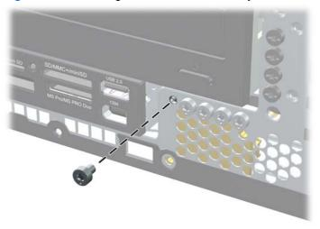
Figure 6-8 Retrieving the Front Bezel Security Screw
